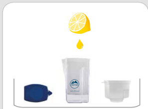
Clean all the reservoirs and parts of the system – but not the two filters – with bio lemon.
